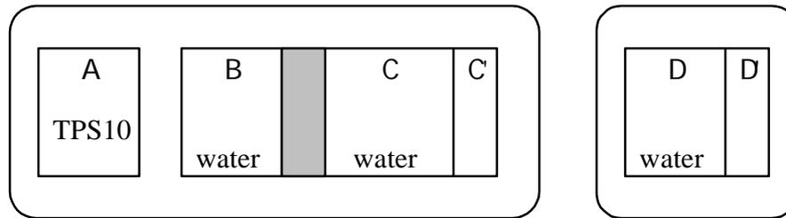
There are totally 4 baths on our Branson ultrasonic cleaner system. They are labeled to be bath A, B, C, and D. C' and D' are the heating baths for bath C and D respectively.
