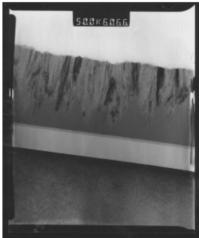
Fig. 6. XTEM micrograph of as-deposited \text{Si}_{0.7}\text{Ge}_{0.3} film at 500^\circ\text{C} on oxidized silicon. The oxide layer is about 100 nm thick. The SiGe film is about 300 nm thick. We can see the 10-nm a-Si deposited during the 30 min of \text{SiH}_4 pretreatment.
