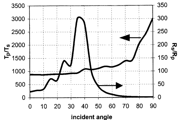
Fig. 6. Reflection and transmission extinction ratios of the WGP as a function of incident angle for the structure S.
