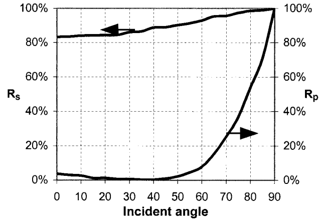
Fig. 5. Reflection of the WGP as a function of incident angle for structure S.
