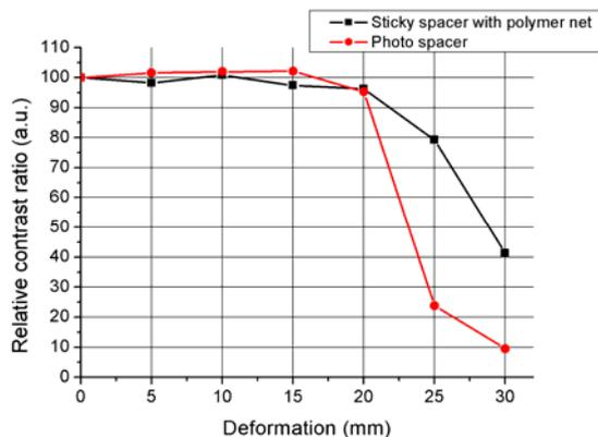
Figure 8: Contrast ratio as a function of bending deformation along the long axis of a smart card with mounted FLC cell.
