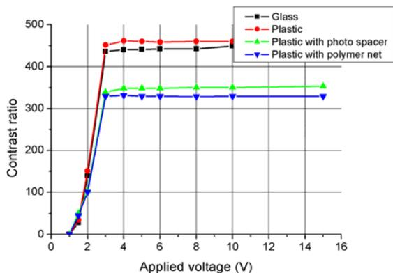
Figure 6: Contrast ratio as a function of applied voltage for the different cell configurations.
