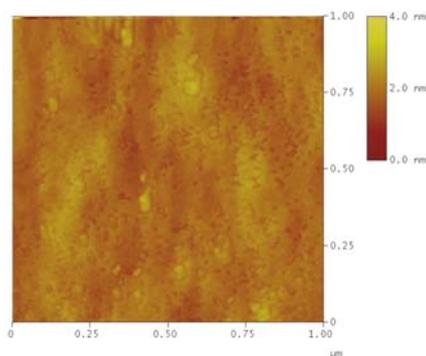
**Figure 3:** AFM picture of uncoated ITO covered PES substrate. The image size is  $1 \times 1 \mu\text{m}^2$  and the height scale is 4 nm.
