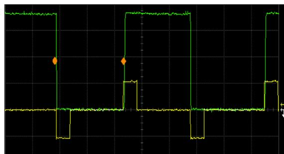
**Figure 5:** Bistable switching of FLC cell on flexible PES substrates.
