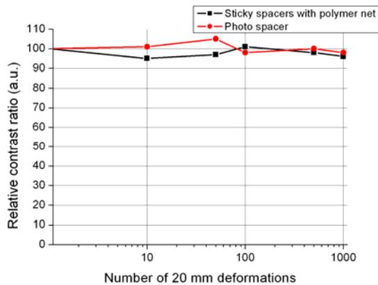
**Figure 10:** Contrast ratio as a function of number of 20 mm deformations along the long axis of a smart card with mounted FLC cell.
