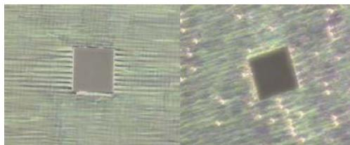
Figure 9: FLC structure before (left) and after (right) severe mechanical deformation of the cell with photo spacers.
