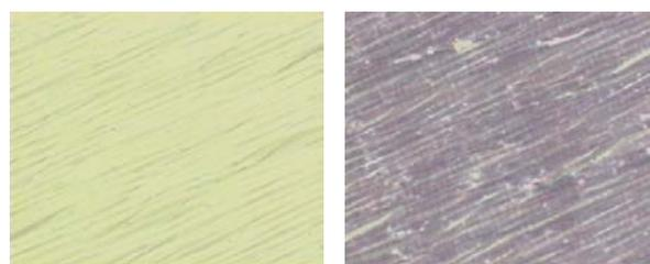
**Figure 4b:** Polarizing microscope images of bright and dark states of glass reference cell. The image size is  $117 \times 142 \mu\text{m}^2$ .
