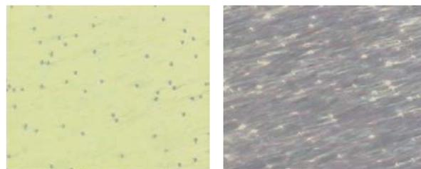
**Figure 4a:** Polarizing microscope images of flexible PES substrate cell. The image size is  $117 \times 142 \mu\text{m}^2$ .
