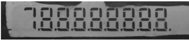
Fig. 12. Photo-aligned 9-digit reflective passive matrix TN-LCD on plastic substrates [37].
