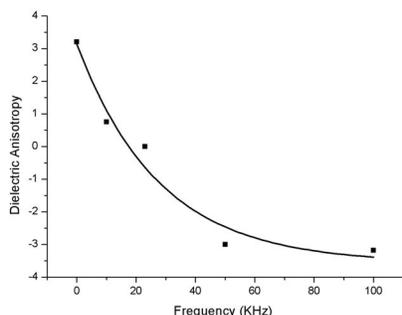
Figure 1. Relationships between Dielectric Anisotropy and Frequency
