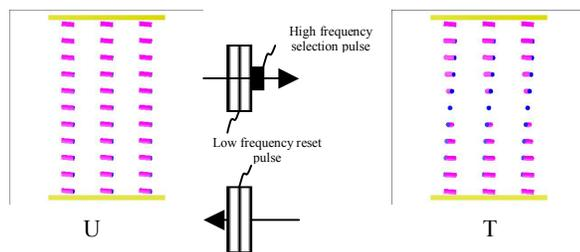
Figure 2. Driving waveform for low (U) and high twist (T) transition.
