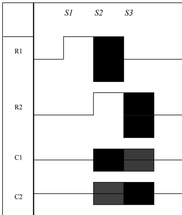
Figure 3. Example of multiplex driving scheme of BTN-LCD.
