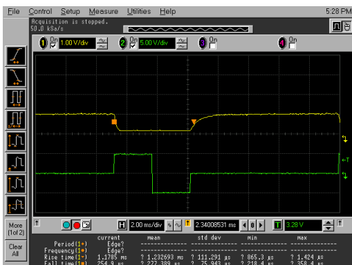
Figure 8 Measured response time of a 4 \mu m NBB test cell.
