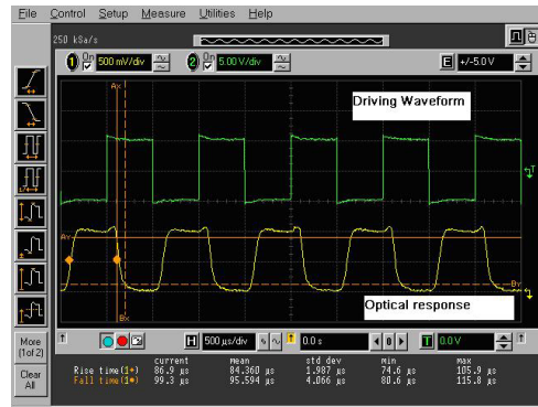
Fig. 3 Electro-optical response without any electrical treatment under binary waveform with V_{am}=5v and T=1ms
