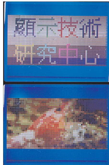
FIGURE 14 — A demonstration unit with 48 \times 64 resolution. Pixel size, 0.5 \times 0.5 \text{ mm} .
