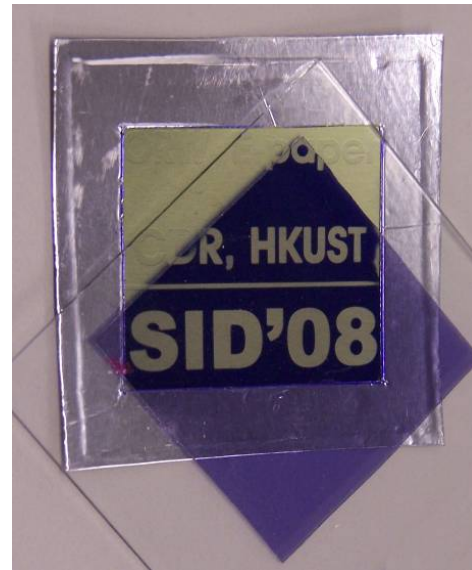
Figure 7. ORW e-paper with fluorescent dye doped LC with top polarizer removed
