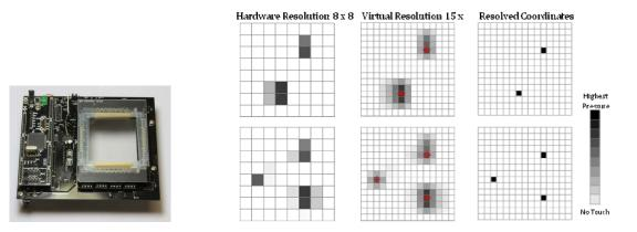
Bilinear interpolation is applied to enhance the resolution by twice. We can further estimate the touch location by analyzing the area and the depth of hotspots. Multiple simultaneous touches can be resolved accurately.
