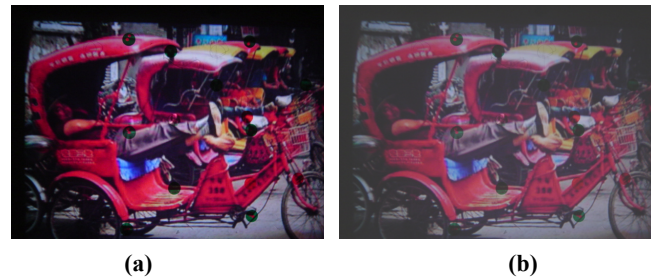
Figure 5 The projection picture from a 0.38" CS-LCOS projector at (a) dimmed light and (b) room light environments
