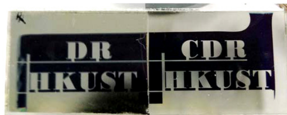
FIGURE 5 — Prototype of the LTN-TN LCD made at the Center for Display Research (CDR).
