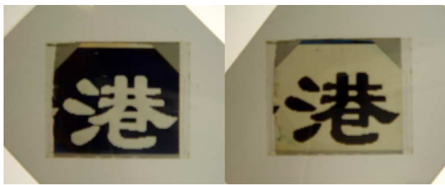
Figure 2. Photo-patterned polarizer. Top: Principal configuration. Bottom: Chinese characters image made by a photo-patterned polarizer.
