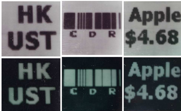
Figure 5. Light printer for optically rewritable E-paper (Top) and the images obtained by optimized STN-LCD mask (Bottom).
